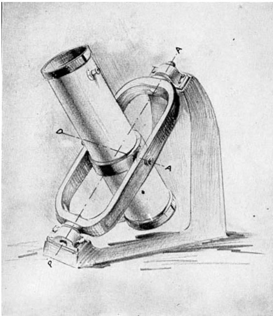
The Double Yoke Equatorial Mounting
