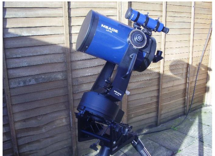
Daran's 200mm SCT Mounted on an Equatorial Wedge
