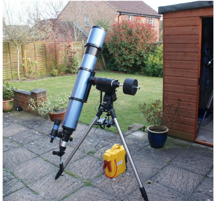
A 120mm Skywatcher Refractor on a EQ5 Mounting
