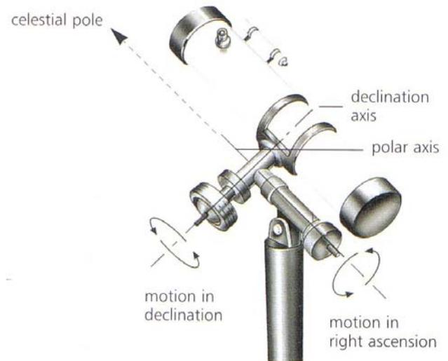
The major advantage of the Equatorial mounting is in its ability to be driven on just one axis to track objects across the sky. By driving the axis with a motor that will give one rotation every 24 hours the telescope will rotate at the same speed as Earth. This type of drive is essential if the telescope is going to be used for photographs or digital imaging with exposure times exceeding 30 seconds.
