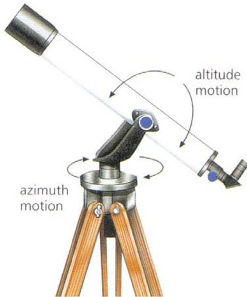
An Alt - Azimuth Mounting
